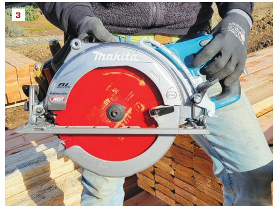
The Makita 40-volt XGT beam saw can cut through 4-by lumber in a single pass (1) and has a large rafter hook that fits over an I-joist (2). The saw has an electric brake to stop the big, 10¼-inch blade (3).
